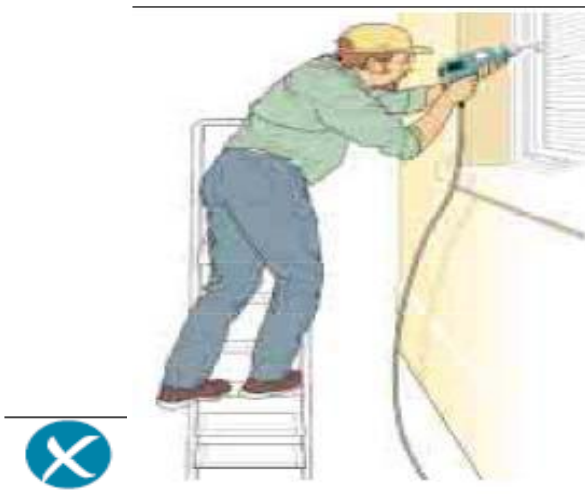
Incorrect – steps side on to work activity
